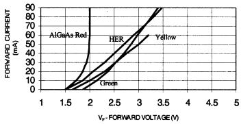
Fig 1. Forward Current vs. Forward Voltage
