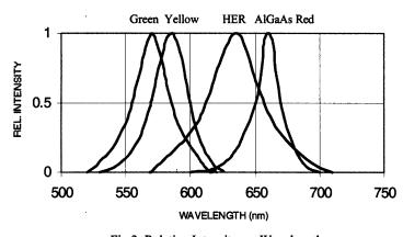
Fig 3. Relative Intensity vs. Wavelength
