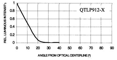
Fig 5. Relative Intensity vs. Angular Displacement
