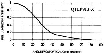
Fig 4. Relative Intensity vs. Angular Displacement
