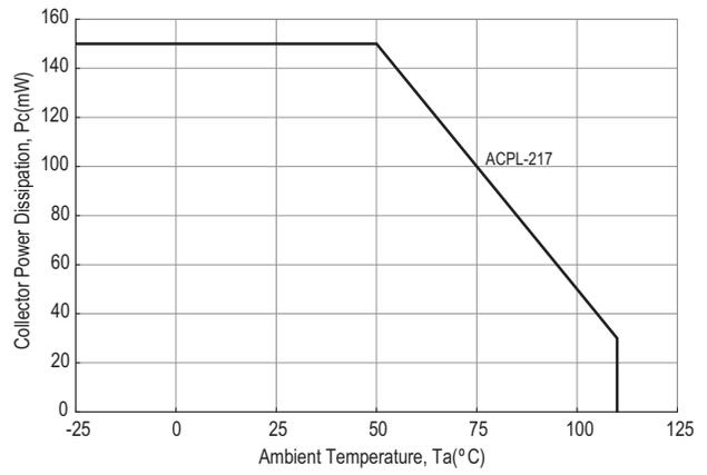
Figure 4. Collector Power Dissipation vs. Ambient Temperature
