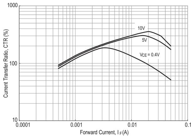
Figure 13. Current Transfer Ratio vs. Forward Current
