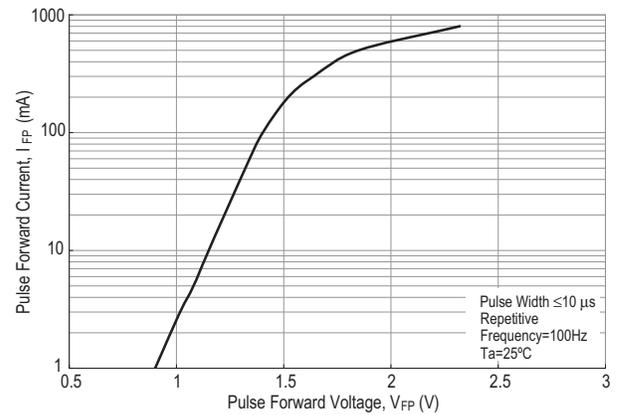
Figure 8. Pulse Forward Current vs. Pulse Forward Voltage
