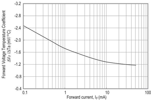
Figure 7. Forward Voltage Temperature Coefficient vs. Forward Current
