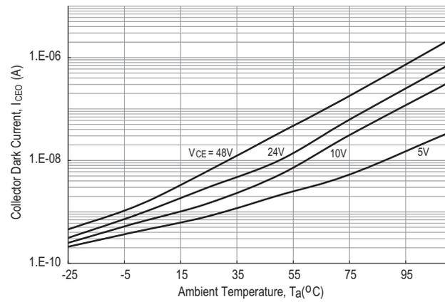
Figure 12. Collector Dark Current vs. Ambient Temperature
