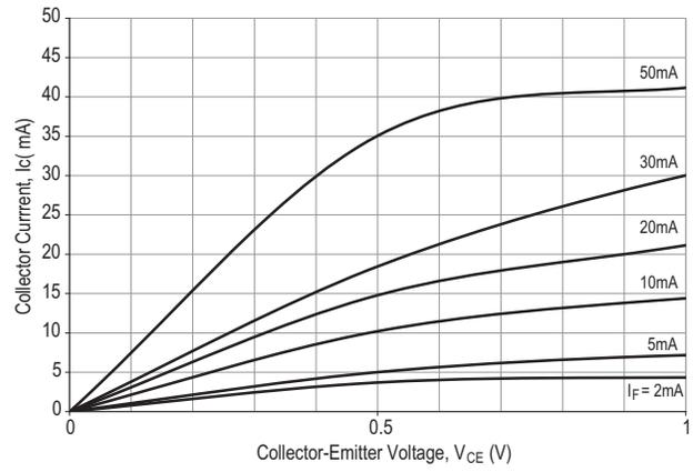
Figure 10. Collector Current vs. Small Collector-Emitter Voltage
