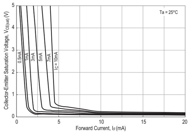
Figure 18. Collector-Emitter Saturation Voltage vs. Forward Current
