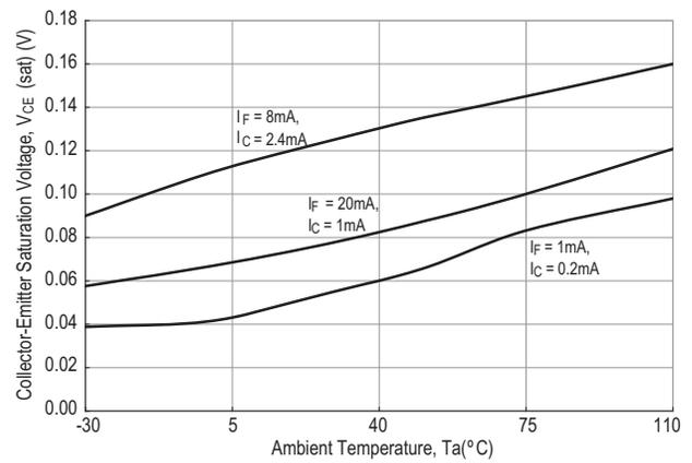
Figure 14. Collector-Emitter Saturation Voltage vs. Ambient Temperature
