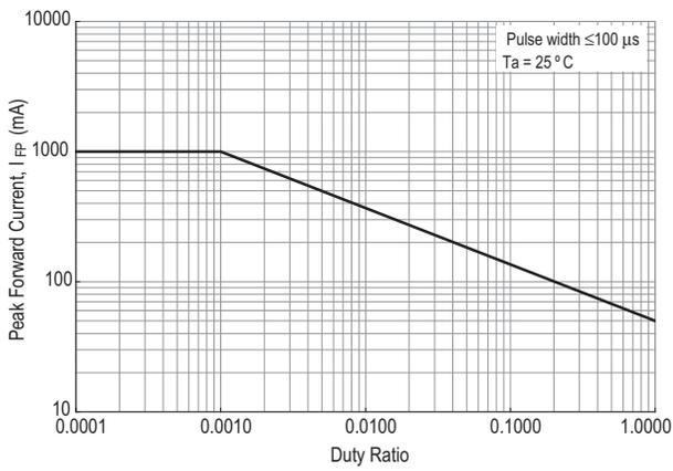
Figure 5. Pulse Forward Current vs. Duty Cycle Ratio
