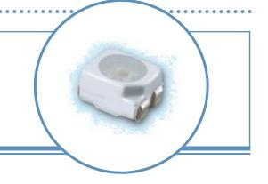
The **OVSAABC2R8** is designed for wide angle, uniform light output. Its internal reflector and colorless clear lens optimize luminous intensity and make it ideal for backlighting applications and for coupling with light guides.
