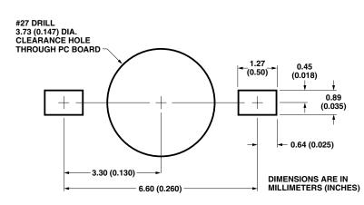
Recommended soldering pad pattern for yoke leads 21, 22, and 24.
