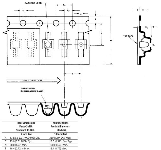
Embossed CarrierAll DimensionsTape DimensionsAre in MillimetersPer ANSI/EIA(Inches).Standard RS-481.
