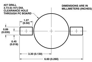
Recommended soldering pad pattern for Z-bend leads 31, 32, and 34.
