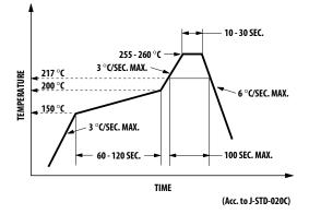
Recommended Pb-free reflow soldering profile.
