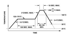
Recommended SnPb reflow soldering profile. Wait until device has cooled to room temperature before handling.
