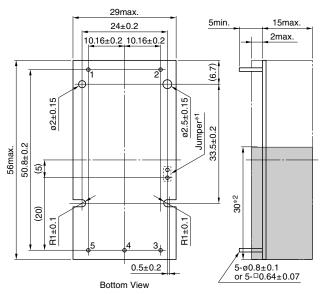
\*1 Terminal numbers 2 and 5 are connected by the jumper. Weight: 21g typ. Cut this jumper to let the secondary side float with respect to the primary side.
