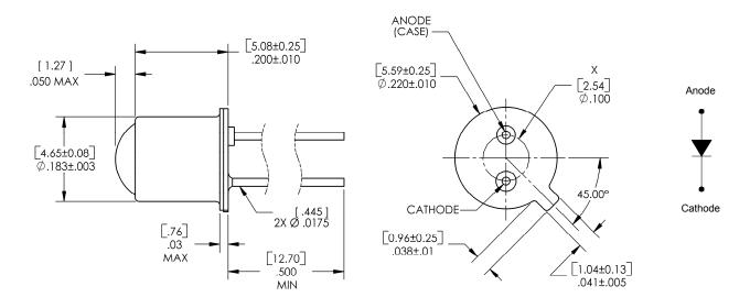
X THIS DIMENSION CONTROLLED AT HOUSING SURFACE.
