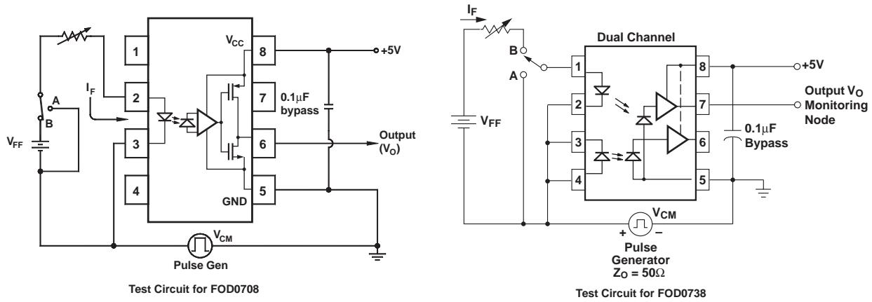
Fig. 11 Test Circuit Common Mode Transient Immunity (FOD0708 and FOD0738)
