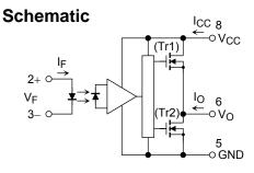
A 0.1  $\mu\text{F}$  bypass capacitor must be connected between pins 8 and 5. (See Note 6)
