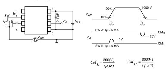
$\mathrm{CM_L}\left(\mathrm{CM_H}\right)$  is the maximum rate of rise (fall) of the common mode voltage that can be sustained with the output voltage in the low (high) state.
