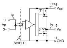
A 0.1  $\mu F$  bypass capacitor must be connected between pin 6 and 4. (See Note 6)
