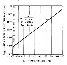
Figure 5. Typical high level supply current,  $I_{\text{CCH}}\,\text{vs.}$  temperature.
