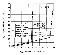
Figure 3. Typical input characteristics, I<sub>IN</sub> vs. V<sub>IN</sub>.
