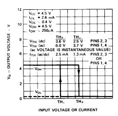
Figure 1. Typical transfer characteristics.
