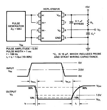
Figure 7. Switching test circuit.
