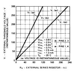
Figure 10. Typical external threshold characteristic,  $V_{\pm}$  vs.  $R_{x}$ .
