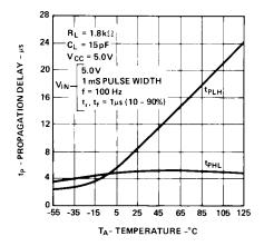
Figure 6. Typical propagation delay vs. temperature.
