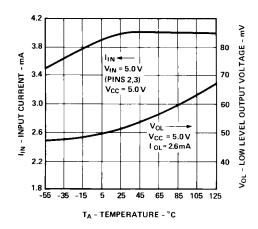
Figure 4. Typical input current,  $\mathbf{I}_{\text{IN}},$  and low level output voltage,  $\mathbf{V}_{\text{OL}},$  vs. temperature.
