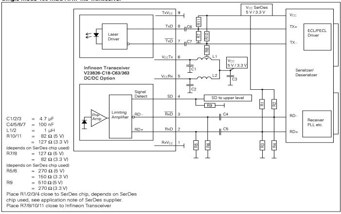
This Application Note assumes Fiber Optic Transceivers using 5 V power supply and SerDes Chips using 3.3 V power supply. It also assumes no self biasing at the receiver data inputs (RD+/ RD-) of the SerDes chip (Refer to the manufacturer data sheet for other applications). 3.3 V-Transceivers can be directly connected to SerDes-Chips using standard PECL Termination network.
