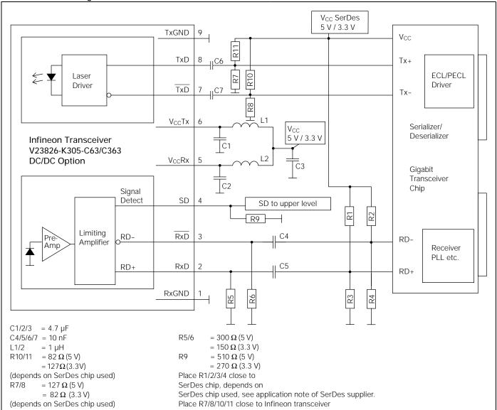
This Application Note assumes Fiber Optic Transceivers using 5 V power supply and SerDes Chips using 3.3 V power supply. It also assumes self biasing at the receiver data inputs (RD+/RD-) of the SerDes chip. Refer to the manufacturer data sheet for other applications. 3.3 V-Transceivers can be directly connected to SerDes-Chips using standard PECL Termination network.
