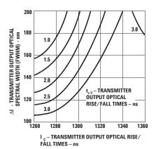
AFBR-5805 TRANSMITTER TEST RESULTS OF I  $_{\rm C}$   $\Delta I$  AND  $_{\rm T/T}$  ARE CORRELATED AND COMPLY WITH THE ALLOWED SPECTRAL WIDTH AS A FUNCTION OF CENTER WAVELENGTH FOR VARIOUS RISE AND FALL TIMES.
