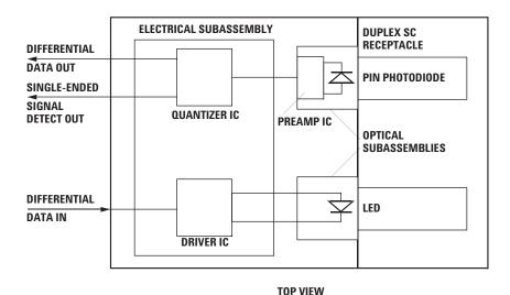
Figure 1. SC Connector Block Diagram
