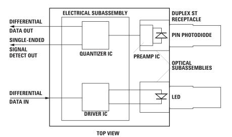
Figure 1a. ST Connector Block Diagram.
