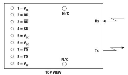
Figure 3. Pin Out Diagram.
