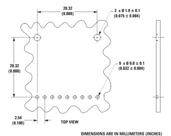
Figure 8. Recommended Board Layout Hole Pattern
