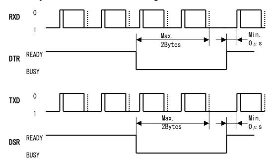
The above timing is RS-232 level. The logical value is inverted from above level.
