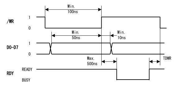
TDWR = Normal command mode: Min 1  $\mu$  S Graphic DMA Mode: Min 15  $\mu$  S
