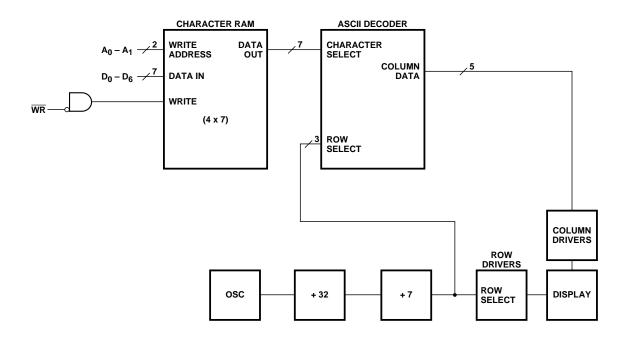
Figure 2. Display internal block diagram.
