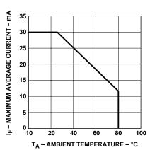
Figure 3. Maximum Allowable Average Current per Dot vs. Ambient Temperature.
