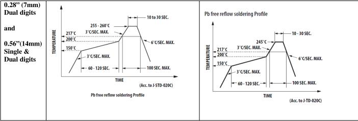
Remarks: The peak temperature refers to the peak temperature measured on the package.
