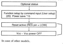
Set the time (tL) from reset active to turning off the VDD - Vss power (VDD - Vss = 1.8 V) longer than the time (th) when the potential of V5 ~ V1 becomes below the threshold voltage (approximately 1 V) of the LCD panel For th, refer to the <Reference Data> of this event. When the is too long, insert a resistor between V<sub>5</sub> and V<sub>DD</sub> to reduce it.
