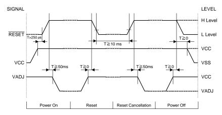
Please maintain the above sequence when turning on and off the power supply of the module. If  $V_{EE}$  and/or  $V_{ADJ}$  is supplied to the module while internal alternate signal for LCD driving (M) is unstable or  $\overline{RESET}$  is active, DC component will be supplied to the LCD panel. This may cause damage to the LCD module.
