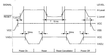
Please maintain the above sequence when turning on and off the power supply of the module. If Vee and/or Vadi is supplied to the module while internal alternate signal for LCD driving (M) is unstable or RESET is active, DC component will be supplied to the LCD panel. This may cause damage to the LCD module.
