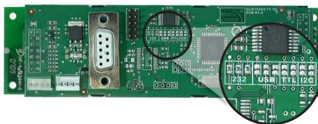
Figure 17: Protocol-Select-Jumpers for GLK19264-7T-1U Non-USB
