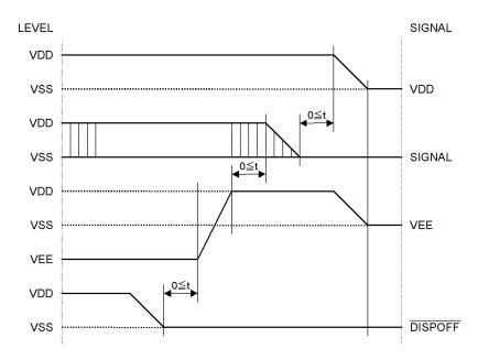
Please maintain the above sequence when turning on and off the power supply of the module
