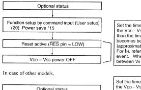
Set the time (tL) from reset active to turning off the VDD - Vss power (VDD - Vss = 1.8 V) longer than the time (th) when the potential of V5 ~ V1 becomes below the threshold voltage (approximately 1 V) of the LCD panel For th, refer to the <Reference Data> of this event. When the is too long, insert a resistor between V<sub>5</sub> and V<sub>DD</sub> to reduce it.
