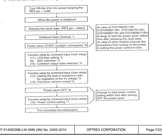
\* The target time of 5ms will result to vary depending on the panel characteristics and the capacitance of the smoothing capacitor. Therefore, we suggest you to conduct an operation check using the actual equipment.
