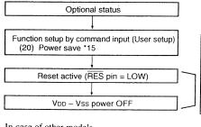
Set the time (t) from reset active to turning off the VDD - Vss power (VDD - Vss = 1.8 V) longer than the time (th) when the potential of V5 ~ V1 becomes below the threshold voltage (approximately 1 V) of the LCD panel. For th, refer to the <Reference Data> of this event. When th is too long, insert a resistor between Vs and Vpp to reduce it.
