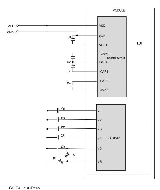
C1~C4: 1.0 $\mu$ F/16V C5~C8: 0.68 $\mu$ F/16V R1: 270K $\Omega$ ±0.2% R2: 1.1M $\Omega$ ±0.2%
