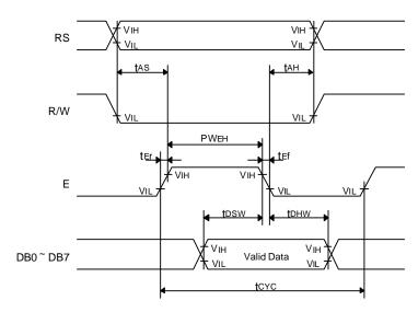
Fig.1 Write Operation Timing
