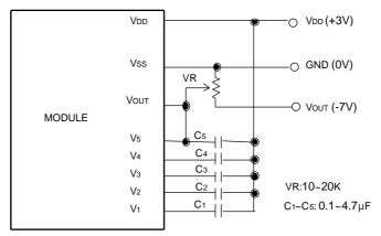
Both the boosting circuit and the voltage control circuit are not used in this module. Therefore, connect V5 pin with Vout pin and supply the LCD driving voltage from the outside.
