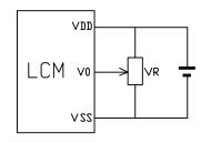
$V_{\text{DD}} \sim V_0$ : LCD Driving voltage
