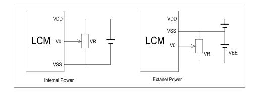
$V_{DD^{\sim}}V_0\text{: LCD Driving voltage}$
