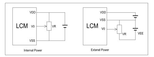
$V_{DD-}V_0$ : LCD Driving voltage VR: 10k~20k
