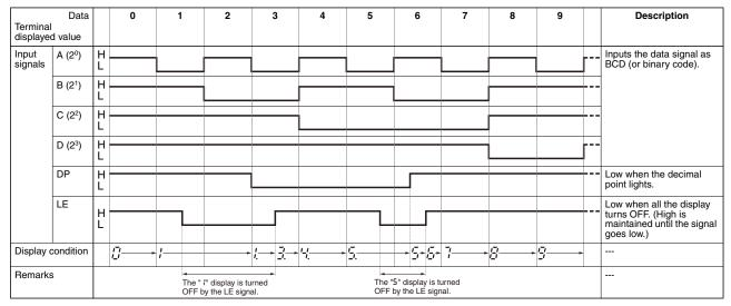
• Using the latch input (LE) terminal for each Unit, the data input terminals (A to D) can be used in common yet still enable display on each Unit (example of a 3-digit dynamic-output model with positive logic).
