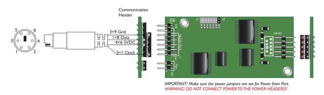
NOTE: Make sure that you have set the jumpers for power-from-port before connecting to the PS/2 port.
