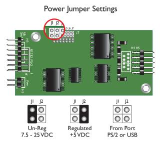
**NOTE:** 5-Wire controller boards are delivered pre-set for USB applications with additional jumpers supplied.
