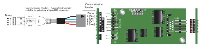
NOTE: Make sure that you have set the jumpers for power-from-port before connecting to the USB port.
