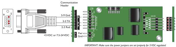
IMPORTANT! Make sure the power jumpers are set properly for 5 VDC regulated or 7.5 - 24 VDC unregulated power before supplying power to the board.
