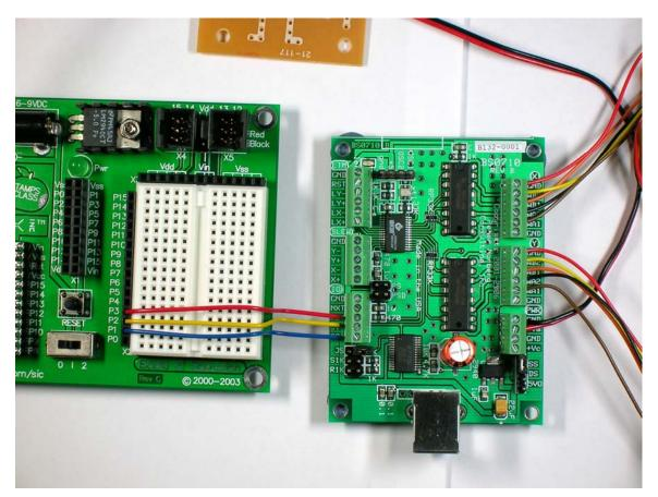
In this case, both boards were powered off of the same 12 volt power source (the BOE can support this without trouble, even though they show 9 volts as the maximum). This allows one power supply to be used to operate both the board logic and the motors themselves.
