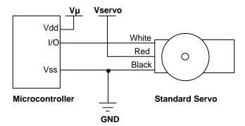
$V\mu$  = microcontroller voltage supply
