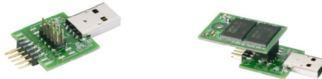
Figure 10: uDiskOnChip 2x5 Horizontal Version, Single/Dual Connector, Top View
