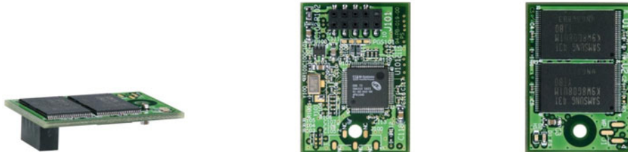
Figure 4: uDiskOnChip Horizontal Version with Single Connector
