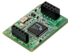
Figure 5: uDiskOnChip Horizontal Version with Dual Connector Configuration
