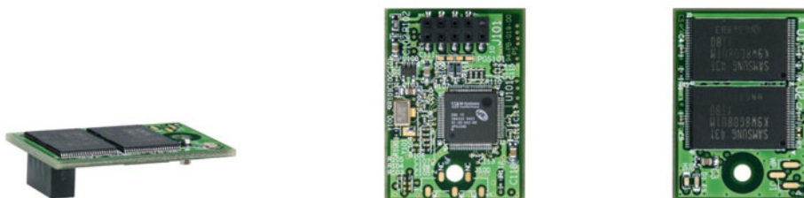
Figure 4: uDiskOnChip Horizontal Version with Single Connector
