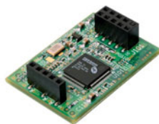
Figure 5: uDiskOnChip Horizontal Version with Dual Connector Configuration
