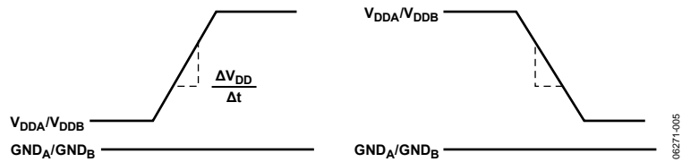
Figure 13. Transient Immunity Waveforms—Output Supplies
