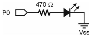
Figure 3.3: Start LED Schematic
