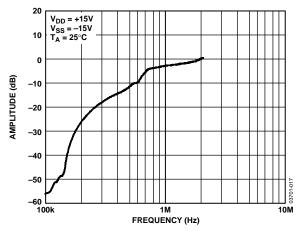
Figure 17. Voltage Sense Amplifier AC PSRR
