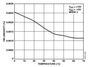
Figure 5. Voltage Sense Amplifier Linearity vs. Temperature
