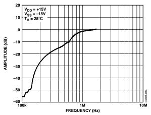
Figure 13. Current Sense Amplifier AC PSRR
