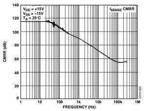
Figure 9. Current Sense Amplifier CMRR vs. Frequency
