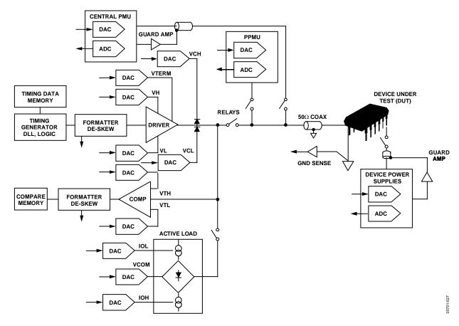
Figure 27. Typical Application ATE Circuit
