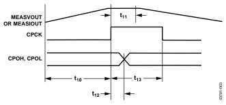
Figure 3. Comparator Timing
