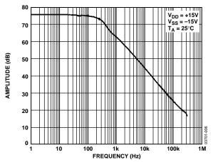
Figure 6. Voltage Sense Amplifier CMRR vs. Frequency
