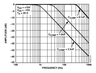
Figure 11. Force Amplifier Bandwidth, Mode 2 (400 μA)
