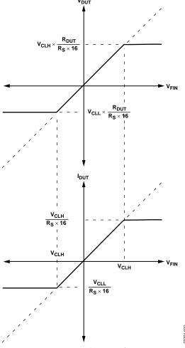
Figure 22. Force Voltage Transfer Function
