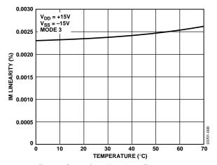
Figure 8. Current Sense Linearity vs. Temperature
