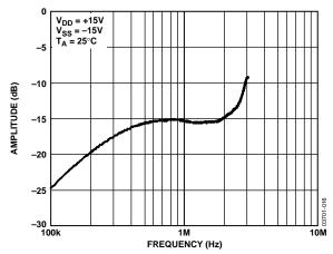
Figure 16. Force Amplifier AC PSRR, Mode 3, C<sub>COMP</sub> = 100 pF
