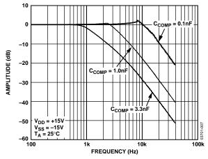
Figure 7. Force Amplifier Bandwidth, Mode 0 (4  $\mu$ A)
