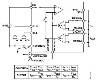
Figure 24. Current Force, Voltage Measure Mode
