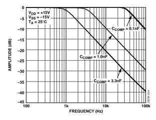
Figure 14. Force Amplifier Bandwidth, Mode 3 (4 mA)
