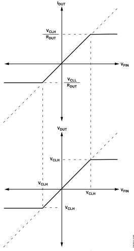
Figure 25. Current Force Transfer Function
