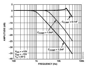
Figure 10. Force Amplifier Bandwidth, Mode 1 (40 μA)
