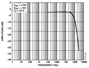
Figure 12. Guard Amplifier Bandwidth
