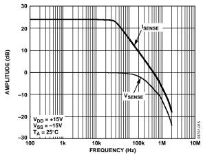
Figure 15. Voltage Sense and Current Sense Amplifier Bandwidths
