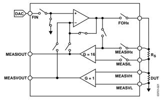
Figure 21. PMU in Standby Mode
