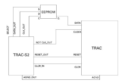
Connections between the support circuit, the EEPROM and the TRAC device are shown above.
