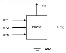
On detecting a switch closure The RF803E will wake up transmit a secure data packet on the TX output.
