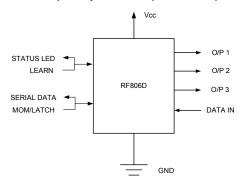
The RF803D is connected directly to the data output of a radio receiver module and upon detection of a valid data packet it will decode the data stream. The RF803D will then assert its digital outputs which will match the state of the RF803E encoders' learnt at the time of transmission.
