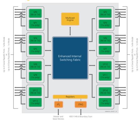
Embedded applications further benefit from the ability to route packets to over 64,000 endpoints through hierarchical lookup tables, independent unicast and multicast routing mechanisms, and error management extensions that provide proactive issue notification to the fabric controller. In addition, the Tsi578 supports both in-band serial RapidIO access and out-of-band access to the full fabric register set through the I<sup>2</sup>C interface.
