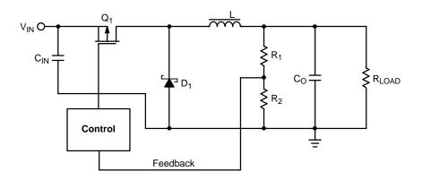
Figure 4. Buck Regulator Block Diagram
