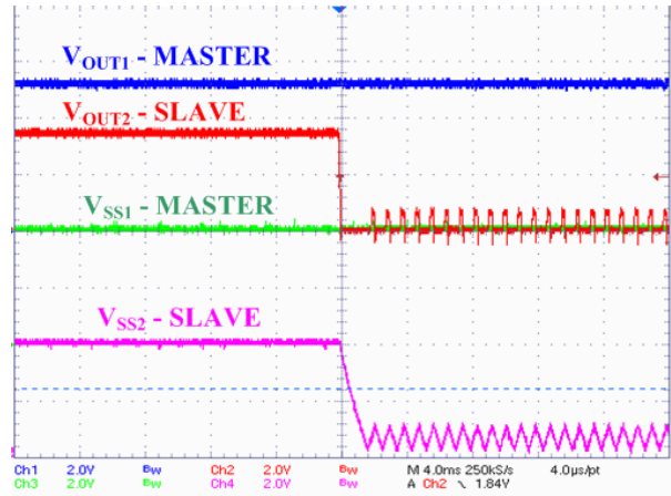
Figure 64. Master Voltage – End of Augmented OLM
