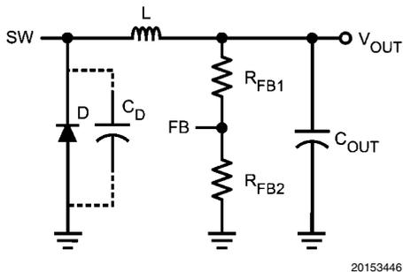
**FIGURE 7. Parasitic Tank Circuit at the Switchpin**
