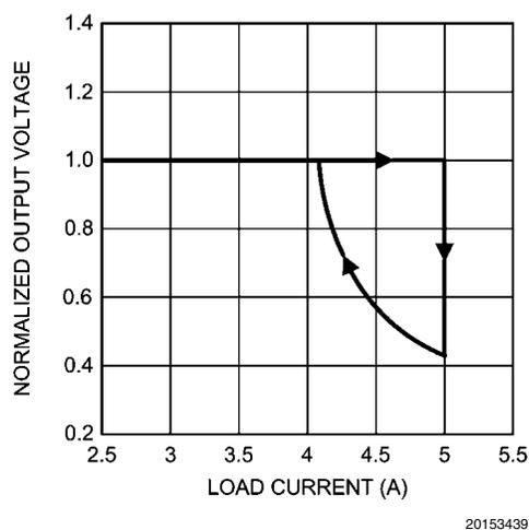
FIGURE 5. Normalized Output Voltage Versus Load Current
