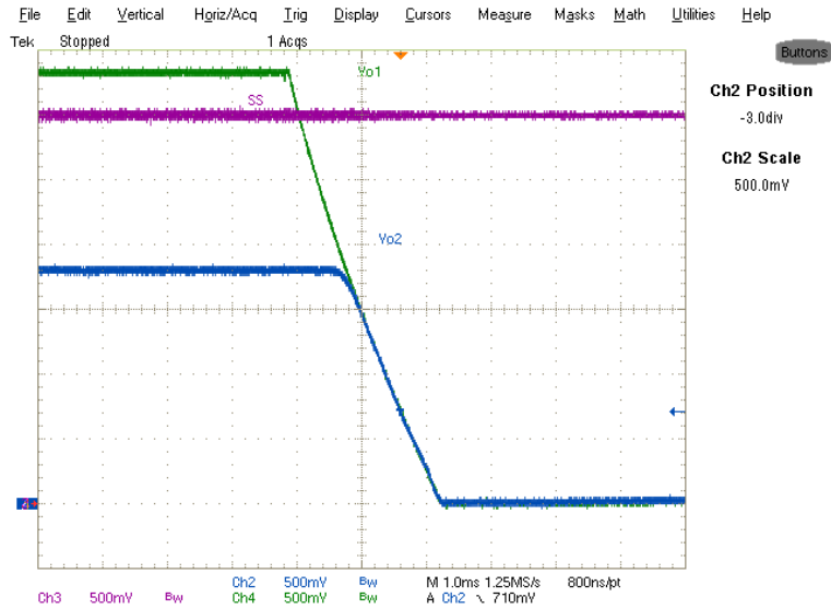
Fig. 25: Simultaneous Tracking a 3.3V input at power-up and shut-down with 6A load. Ch 2 : Vo 2 (1.8Vout) Ch 3 : SS(1.8V) Ch 4 : Vo 1 (3.3V)
