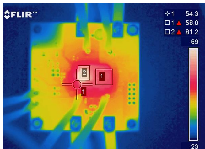
Figure 16: Thermal Image at I_{OUT} = 12A (IR3876: 81^\circ C , Inductor: 58^\circ C , PCB: 54^\circ C )
