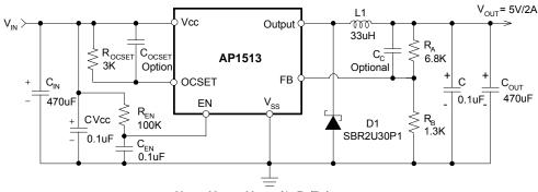
Note:  $V_{OUT} = V_{FB} \times (1+R_A/R_B)$  $R_B = 0.7K \sim 5K \text{ ohm}$
