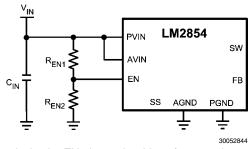
Alternatively, the EN pin can be driven from another voltage source to cater for system sequencing requirements commonly found in FPGA and other multi-rail applications. The following schematic shows an LM2854 that is sequenced to start based on the voltage level of a master system rail.
