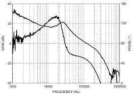
$\begin{array}{c} \text{LM2854 500 kHz Bode Plot} \\ \text{V}_{\text{IN}} = 5.0\text{V}, \text{V}_{\text{OUT}} = 1.8\text{V}, \text{I}_{\text{OUT}} = 4\text{A} \\ \text{R}_{\text{FB1}} = 250 \text{ k}\Omega, \text{R}_{\text{COMP}} = 1 \text{ k}\Omega, \text{C}_{\text{COMP}} = 47 \text{ pF}, \\ \text{L}_{\text{OUT}} = 1.5 \text{ \muH}, \text{C}_{\text{OUT}} = 100 \text{ \muF ceramic} \end{array}$
