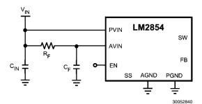
In general,  $R_F$  is typically selected between  $1\Omega$  and  $10\Omega$  so that the steady state voltage drop across the resistor due to the AVIN bias current does not affect the UVLO level. Recommended filter capacitor,  $C_F$ , is 1.0  $\mu F$  in X5R or X7R dielectric.
