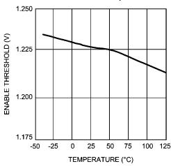
**Enable Threshold vs. Temperature**
