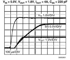
LM2854 500 kHz Power On via Enable  $V_{\rm IN}$  = 5.0V,  $V_{\rm OUT}$  = 1.8V,  $I_{\rm OUT}$  = 4A,  $C_{\rm SS}$  = 220 pF
