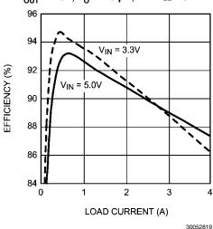
LM2854 1 MHz Efficiency vs.  $I_{OUT}$  V $_{OUT}$  = 2.5V,  $L_{O}$  = 1.0  $\mu$ H, 7.1  $m\Omega$  DCR
