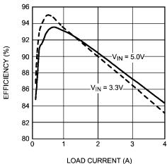
LM2854 500 kHz Efficiency vs. I<sub>OUT</sub>
