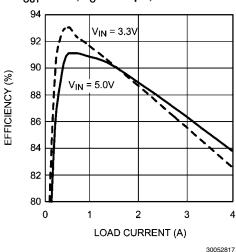
LM2854 1 MHz Efficiency vs.  $I_{OUT}$  V  $_{OUT}$  = 1.8V,  $L_{O}$  = 1.0  $\mu$ H, 7.1  $m\Omega$  DCR
