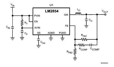
TABLE 5. LM2854 500kHz Bill of Materials,  $V_{IN}$  = 5V,  $V_{OUT}$  = 3.3V,  $I_{OUT(MAX)}$  = 4A, Optimized for Efficiency
