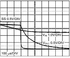
LM2854 1 MHz Load Transient Response  $V_{IN}$  = 5.0V,  $V_{OUT}$  = 3.3V,  $I_{OUT}$  = 0.5A to 4A to 0.5A step di/dt  $\cong$  4A/µs,  $C_O$  = 100 µF ceramic
