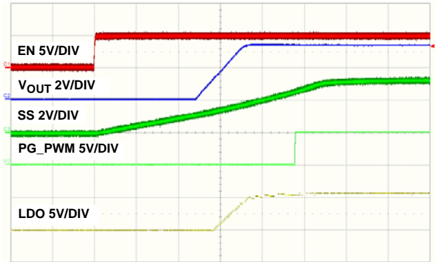
FIGURE 21. SOFT-START AT NO LOAD, 500 \mu s/DIV
