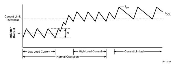
FIGURE 4. Inductor Current - Current Limit Operation
