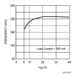
FIGURE 8. Frequency vs V<sub>IN</sub> Circuit of *Figure 6*
