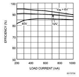
FIGURE 7. Efficiency vs Load Current and V<sub>IN</sub>
