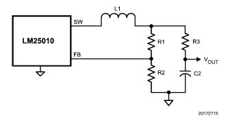
FIGURE 9. Low Ripple Output
