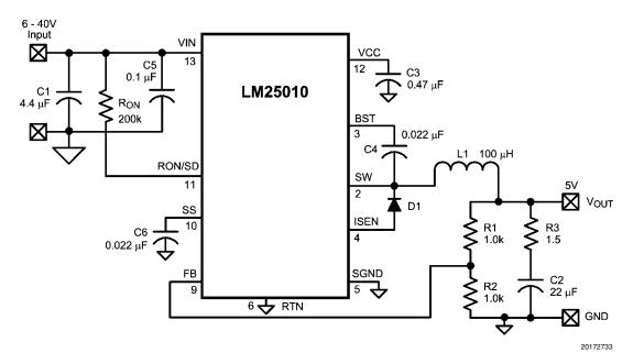
FIGURE 6. Example Circuit
